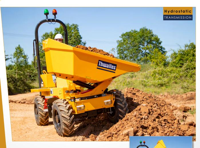
The Thwaites 2.3 Tonne Power Swivel, Stage V dumper is manufactured with contractors and hirers in mind – ensuring operator safety, reducing risk on site and improving performance. Powered by an 18.1 kW 3-cylinder Yanmar engine, delivering 107 Nm max torque for optimum traction and control, this machine is driven by a Hydrostatic transmission, making it simple and straightforward to operate.
